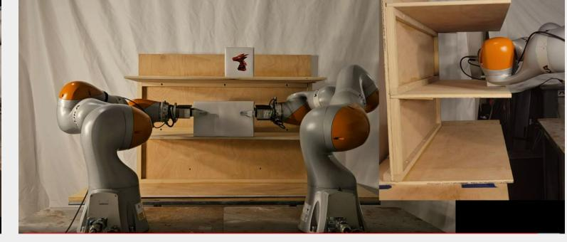
Moving boxes of different sizes between a set of shelves with the Graph of Convex Sets planner.
